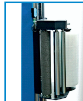
- Option 1: Cutting Unit (Cutting film after ending wrapping)
