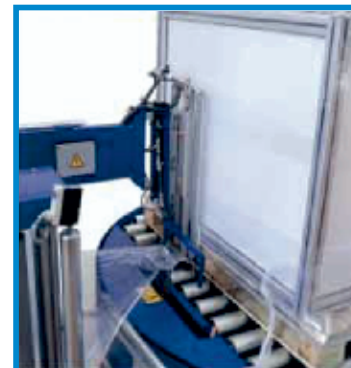
- Option 1: Cutting Unit (Cutting film after ending wrapping)
